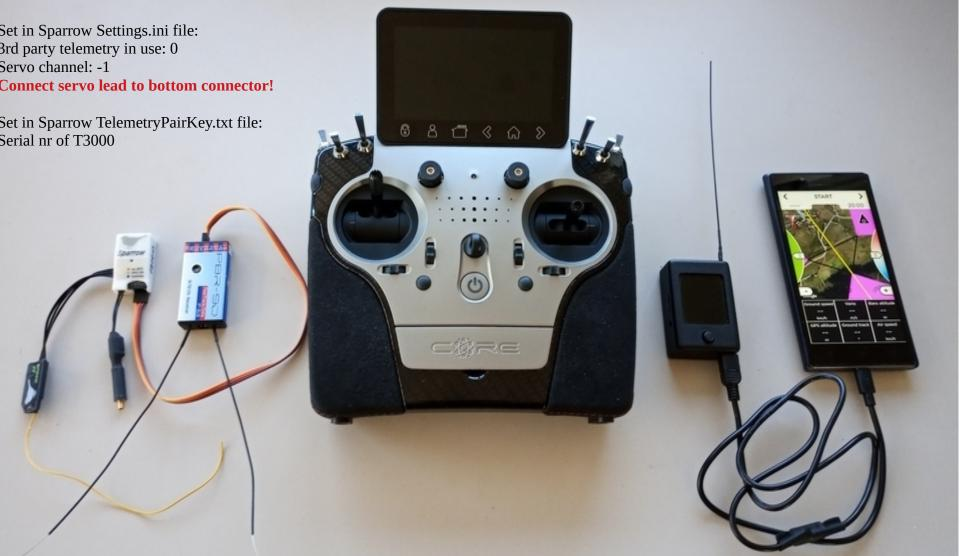
Set in Sparrow Settings.ini file: 3rd party telemetry in use: 0 Servo channel: -1 **Connect servo lead to bottom connector!**
